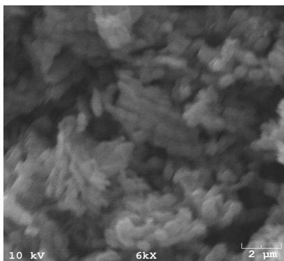
Fig. 4. SEM photograph of CMK-3.
