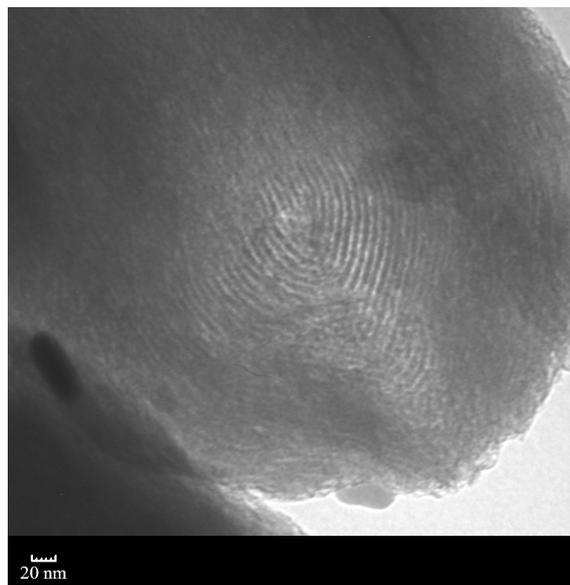
Fig. 5. TEM image of mesoporous carbon material.
