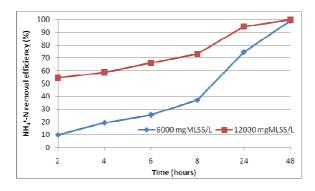
Figure 7. Effect of MLSS on removal ammonium.
