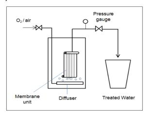
Figure 1. Schematic of the submerged membrane bioreactor system.
