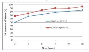
Figure 8. Effect of MLSS concentration on T-P removal efficiency.
