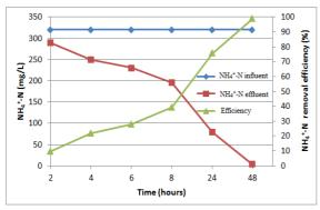
Figure 4. Effect of HRT on removal ammonium.
