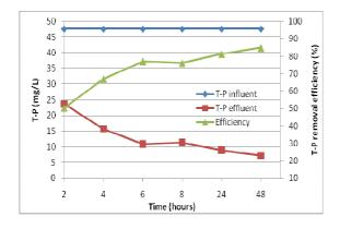
Figure 5. Effect of HRT on T-P removal efficiency.
