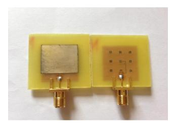
a) A microtrip antenna and a meta-antenna.
