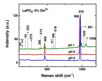
Fig. 5. Room temperature Raman spectra of  $LaPO_4$  nanopowders prepared at pH = 1, 6, and 9.
