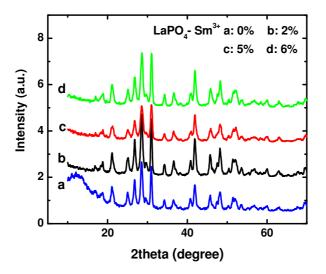
Fig. 3. XRD patterns of LaPO<sub>4</sub>:Sm<sup>3+</sup> (0, 2, 5, and 6 mol%) nanowires prepared at 220 °C for 6 h.
