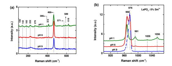
Fig. 6. Room temperature Raman spectra of the LaPO<sub>4</sub> nanopowers prepared at pH = 1, 6, and 9 in various wavenumber region (a) from 100 cm<sup>-1</sup> to 700 cm<sup>-1</sup> and (b) from 900 cm<sup>-1</sup> to 1080 cm<sup>-1</sup>.
