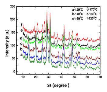
Fig. 2. XRD patterns of LaPO<sub>4</sub> nanowires prepared at hydrothermal temperatures of  $120 - 220^{\circ}$ C for 6 h.
