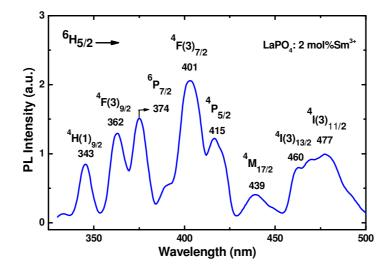
Fig. 11. PLE spectrum monitored at 596 nm of LaPO<sub>4</sub>:Sm<sup>3+</sup> (2 mol%) nanowires.
