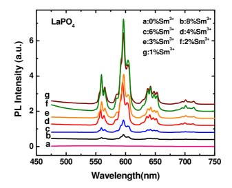
Fig. 9. PL spectra of LaPO<sub>4</sub>:  $Sm^{3+}$  (0, 1, 2, 3, 4, 6, 8 mol%) under 401 nm excitation wavelength.
