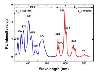
Fig. 8. Typical PL and PLE spectra of LaPO<sub>4</sub>:Sm<sup>3+</sup> (2 mol %) nanowires.
