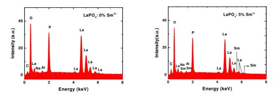
Fig. 7. The EDS spectra of LaPO<sub>4</sub> and LaPO<sub>4</sub>:Sm<sup>3+</sup> (5 mol%) nanowires prepared at 220 °C for 6 h.
