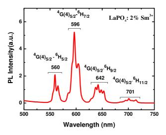
Fig. 10. PL spectrum of LaPO<sub>4</sub>: Sm<sup>3+</sup> (2 mol%) nanowires under 403 nm excitation wavelength.
