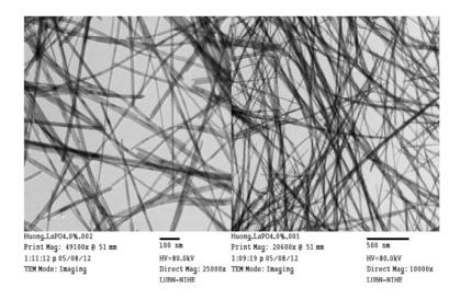
Fig. 1. TEM image of LaPO<sub>4</sub> nanowires synthesized at 220°C for 6 h.
