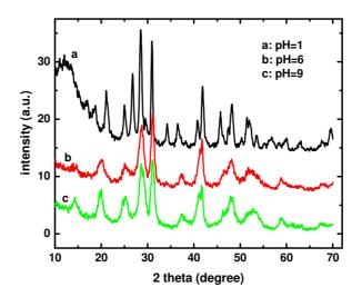
Fig. 4. XRD patterns of the undoped LaPO<sub>4</sub> nanowires prepared at pH = 1, 6, and 9.
