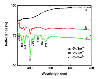
Fig. 12. Diffuse reflection spectra at room temperature of the LaPO<sub>4</sub>:Sm<sup>3+</sup> (0, 2, 6 mol%) nanowires.
