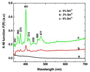
Fig. 13. Plot of Kubelka-Munk function F(R) proportional to absorption coefficient for the LaPO<sub>4</sub>:Sm<sup>3+</sup> (0, 2, 6 mol%) nanowires.
